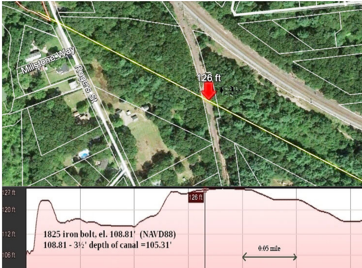
Figure 2.6-5: Elevation Profile of Former Canal Path Prior to Blasting at the “Deep Cut”
